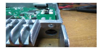
We then took our cable and stripped 4" from one end, fed it through the hole and secured it with a tie wrap:
