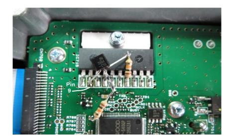
Solder one end of the other 10K resistor to pin 4 of IC715 and the other end to the collector of the NPN transistor. This junction will be your COS signal to the RC210.
