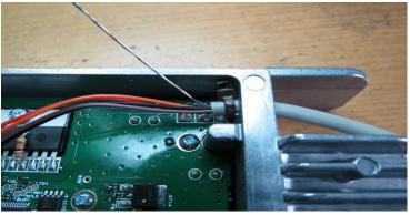
Cut the shield wire to about 2" and slide some heat shrink tubing over it and solder to the point shown.
