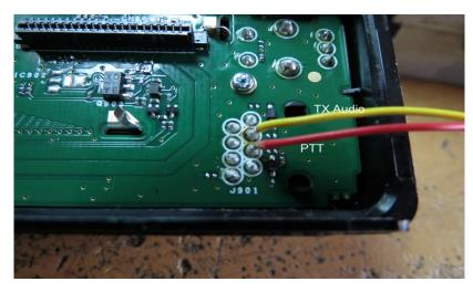
Carefully place the front panel near the chassis, reconnect the flat ribbon cable you removed in the previous step, route the 2 new wires through the opening and snap the front panel back onto the chassis of the radio.
