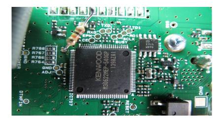
Now take your NPN transistor, bend the leads as shown, lay over IC715 (the AF Amplifier IC) and solder the emitter lead to pin 9. Solder the other end of the 10K resistor you used in the previous step to the base of the NPN transitor.
