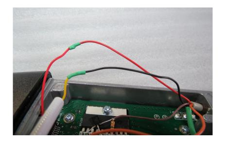
And finally, solder the remaining wire in your 4 conductor cable to the transistor/collector junction for your COS out signal. In our case, we used the brown wire.
